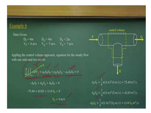
So, numerically that is what is coming. For the steady flow this becomes zero. So, you have in and out. As you know, this in will be negative and both out will be positives, and substituting these Q values for all the cases, with  $V_R$  unknown. So finally, substituting to this equations will give  $V_R$  equal to 4 m/s. So, very simple form of solving the pipe problems where you have one inlet and two outlets.
