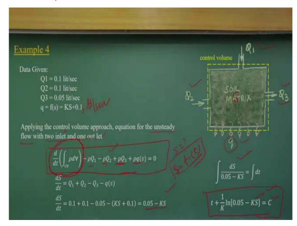
Now, I have to simplify the problem. I have to apply under this control volume the basic mass conservation equations. It is unsteady equation with two inlets and one outlet. That is what you can do, Q1 and Q2 are inlets, Q3 is outlet. Then, the outlet is a seepage part which is going out which will be in terms of S. If you look, when I consider this is the control volume having Q1, Q2, the inflows, and Q3 is outflow, and q is also outflow, which is a functions with respect to S, the storage.
