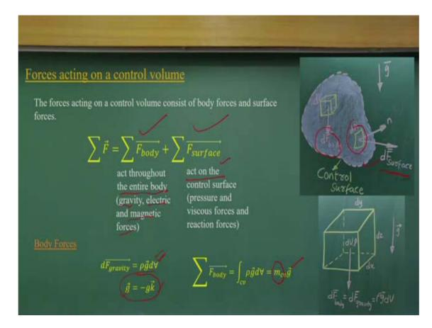
Now, let us come to derive the linear momentum equations, okay? So, we are going for solving these flow problems for linear momentum equations. That means we will consider the control volumes, we have considered the control volume like this. So, each control volume has the control surface. It could be a very simple tetrahedral type of structure or you can have very complex, it does not matter what could be the shapes, okay?
